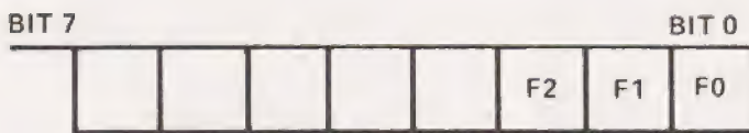
Fig. 5. The status register of a microprocessor. The flag locations are the three least significant bits.
